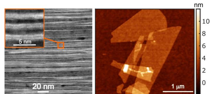
**Fig. 1.** (Left) An image showing the cross-section layered structure of  $H_xCrS_2$ . (Right) An image of the exfoliated nanosheets with a thickness of 2-3 nm.
