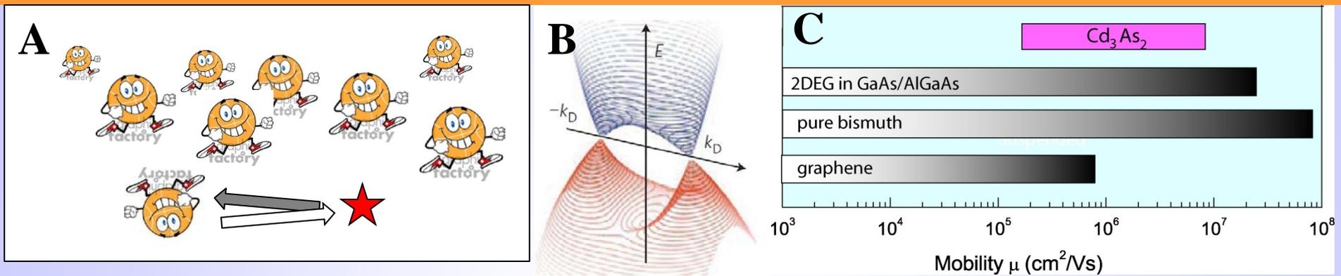
Figure (A) Back scattering of electrons degrades mobility. (B) Schematic of the dispersion of the bulk Dirac states in Cd<sub>3</sub>As<sub>2</sub>. (C) Comparison of the mobilities (at 4 K) in Cd<sub>3</sub>As<sub>2</sub>, the 2DEG in GaAs/AlGaAs quantum wells, in pure bismuth and graphene.
