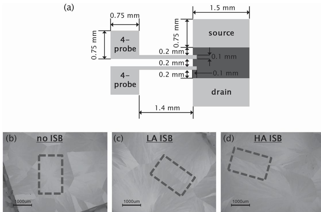
**Figure 1.** a) Electrode geometry for gated four-probe measurements. The shadow mask was aligned to have an ISB running across the channel between the four-probe voltage electrodes for devices comprising an LA and an HA ISB. The highlighted area in (a) is the active channel of the device. The channel areas of devices b) within a single spherulite (i.e., no ISB), c) comprising an LA ISB, and d) an HA ISB are outlined in the optical micrographs.
