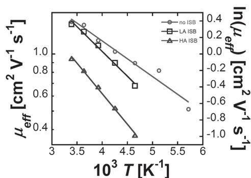
**Figure 3.** Arrhenius plot of the effective mobilities,  $\mu_{\text{eff}}$ , extracted from gated four-probe variable temperature,  $T$ , measurements performed within a single spherulite (circles), across an LA ISB (squares), and across an HA ISB (triangles). All mobilities were extracted at  $V_G = V_T - 25$  V, that is, at the same concentration of mobile carriers. The solid lines are the linear fits used to calculate the activation energy,  $E_A$ , in each case using Equation (2).
