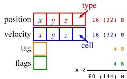
**Fig. 2.** Particle data and memory requirements (in bytes) per MPCD particle. Each particle property is stored in a separate array. Position and velocity arrays are four-element vectors of 32-bit (or 64-bit) floating-point values, and tag and flag arrays are 32-bit integers. A duplicate is allocated for each array to facilitate sorting indicated by  $\times 2$ .
