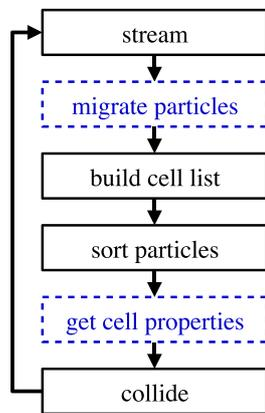
**Fig. 1.** Flow diagram of a single step of the MPCD algorithm. Each block represents an independent step of the algorithm. Blocks with dashed outlines require nearest-neighbor MPI communication for multi-GPU simulations. Particle sorting is an optional step that is performed periodically.
