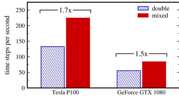
Fig. 6. Time steps per second for SRD collision rule in double precision and mixed precision on NVIDIA Tesla P100 and GeForce GTX 1080 GPUs for the  $L = 100 a$  simulation box.
