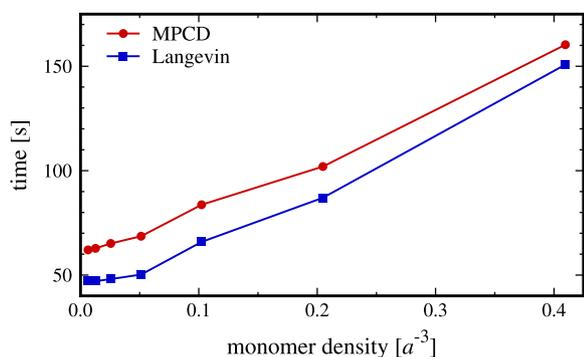
**Fig. 10.** Required time to simulate polymer solutions at various concentrations for  $2000 \tau$  using MPCD (circles) and Langevin dynamics (squares) on an NVIDIA Tesla P100 GPU.
