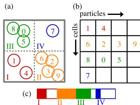
**Fig. 3.** (a) Schematic illustration of particles binned into MPCD cell list. (b) Two-dimensional row-major layout of cell list with one row per cell and columns containing particles. (c) One-dimensional cell list memory with numbers indicating region for each cell and white space showing unused storage per cell.
