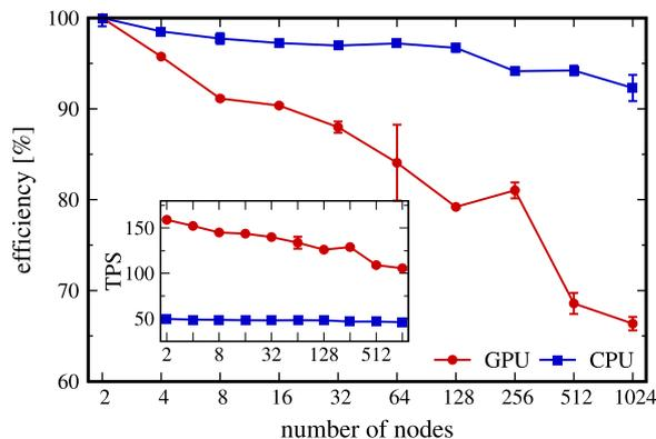
**Fig. 7.** Weak scaling efficiency for benchmark SRD fluid on NCSA Blue Waters. One cubic simulation box with  $L = 50 a$  was replicated per node so that there were 1,250,000 particles per node on average. GPU benchmarks (circles) were performed using 1 MPI rank (1 NVIDIA Tesla K20x GPU) per XK7 node, while CPU benchmarks (squares) used 16 MPI ranks (16 floating-point cores) per XE6 node. The inset shows the performance in time steps per second (TPS).
