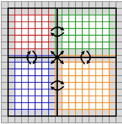
**Fig. 4.** Schematic of MPCD cells with domain decomposition. The global and local simulation box boundaries are indicated by solid black lines. Cells requiring communication, including ghost cells outside global simulation box, are shaded gray. Arrows schematically illustrate the point-to-point MPI communication pattern with neighboring ranks used in both particle migration (Section 3.3) and cell property calculation (Section 3.5) for the GPU.
