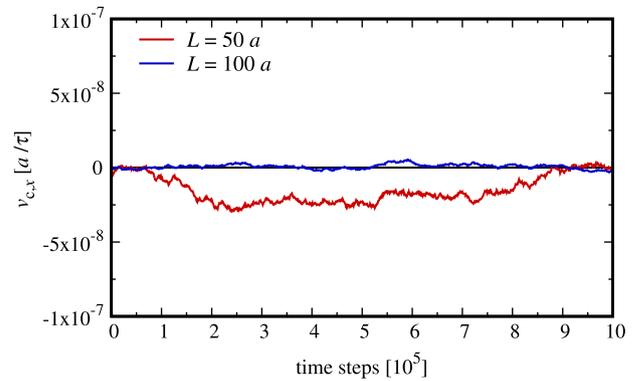
Fig. 5. Center-of-mass velocity of benchmark SRD fluid along  $x$  direction,  $v_{c,x}$ , in mixed-precision model over  $10^6$  MPCD time steps for box sizes  $L = 50 a$  and  $100 a$ .
