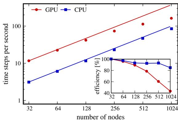
**Fig. 8.** Strong scaling performance for benchmark SRD fluid in a cubic simulation box with  $L = 400 a$  on NCSA Blue Waters. The total number of particles was  $N = 640,000,000$ . GPU benchmarks (circles) were performed using 1 MPI rank (1 NVIDIA Tesla K20x GPU) per XK7 node, while CPU benchmarks (squares) used 16 MPI ranks (16 floating-point cores) per XE6 node. Solid lines indicate ideal scaling, and the inset shows the strong scaling efficiency.
