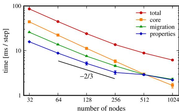
**Fig. 9.** Profile of GPU strong scaling for SRD fluid on NCSA Blue Waters (see Fig. 8). Required time per step is shown for the total simulation (circles), core SRD methods (squares), particle migration (triangles), and computing cell properties (diamonds). Solid black line indicates ideal scaling of the cell property communication.
