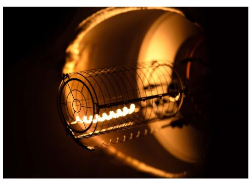
Viewing of an electron emission filament in the CreaTec low-temperature, high-vacuum scanning probe microscope. This system provides a combined in-situ capability of both non-contact atomic force microscopy and scanning tunneling microscopy imaging at single atom scale.
