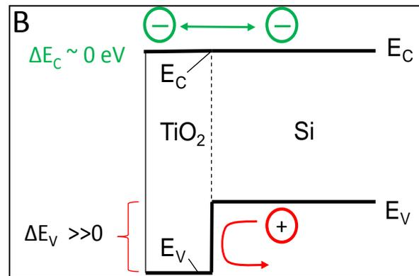
Fig. 1A The energy band edges  $E_c$  and  $E_v$  in P3HT/Si heterojunction. When the highest occupied band (HOMO) of P3HT is aligned with  $E_v$  in Si, electron flow is blocked, but holes are transmitted. Panel 1B shows hole blocking in the complementary  $\text{TiO}_2$ /Si heterojunction.
